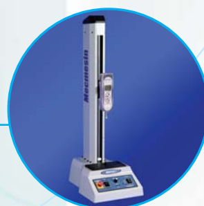
AFG mounted on MultiTest 1 stand
