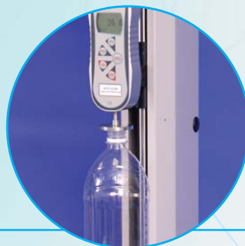
PET bottle top-load test, using an AFG with MultiTest 1 motorised test stand
