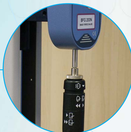
BFG testing automotive stalk
